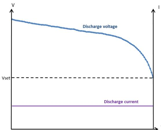
The PSU uses the constant current mode to discharge the battery, and the sink current cannot be set in the discharge mode. During the discharge process, the output voltage will continue to drop to around  $V_{set}$ .
