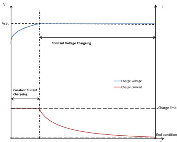
**Constant current stage:** In the initial stage, the PSU charges the battery with the Charge limit, and the output voltage continues to increase to nearly equal to  $V_{set}$ .
